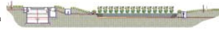
Section of the designed constructed wetland to treat part of the wastewater of Toscanella
